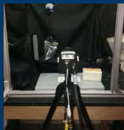
Figure 2: PIV capture setup
