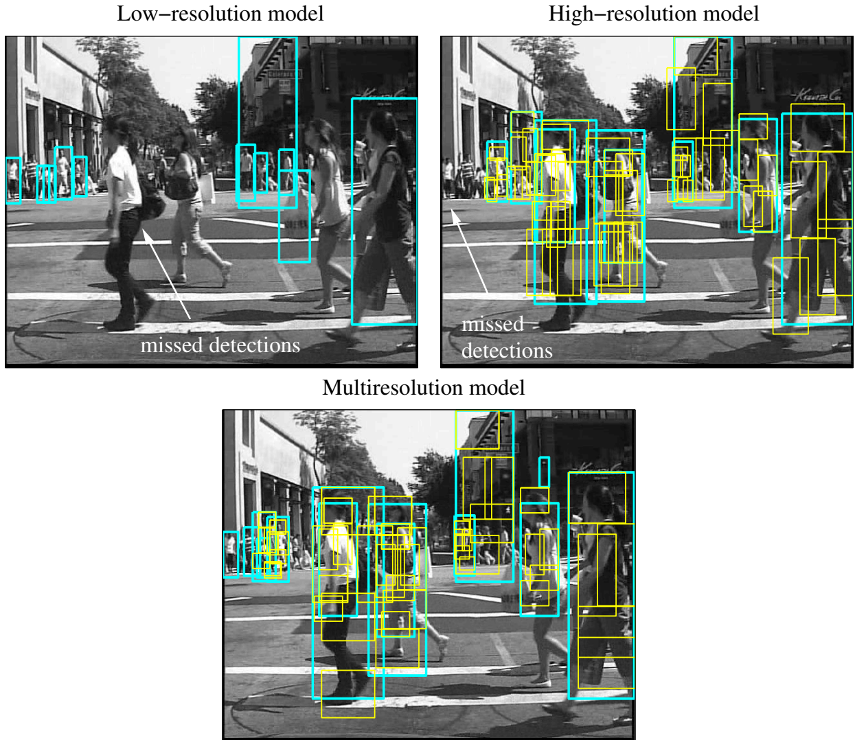
Figure 2.3: On the left , we show the result of our low-resolution rigid-template baseline. One can see it fails to detect large instances. On the right , we show detections of our high-resolution, part-based baseline, which fails to find small instances. On the bottom , we show detections of our multiresolution model that is able to detect both large and small instances. The threshold of each model is set to yield the same rate of FPPI of 1.2.
