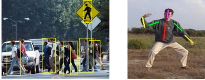
Figure 1.1: Human detection and pose estimation. The simplest type of understanding human in imagery is to detect human as a blob . A standard representation is a rectangular bounding box encapsulating the body ( left ). A higher level understanding is based on pose estimation, which is typically represented by 2D coordinates of body joints ( right ).
