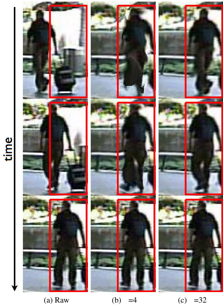
Figure 3.2: Stabilization using coarse-scale LK flows. We show temporally distant 3-frame sequences stabilized onto the last frame (bottom row). The red box in each frame is the location of the person in the last frame. (a) In the raw video, the person shifts from left to right due to camera and object motion. (b) Using fine-scale LK flows, the overall body is stabilized onto the last frame at the cost of distortion in body parts (most visible at the heads and legs of the top row). (c) Using coarse-scale LK flows the warped images are aligned in terms of the overall body location while still preserving clear motions of body parts.
