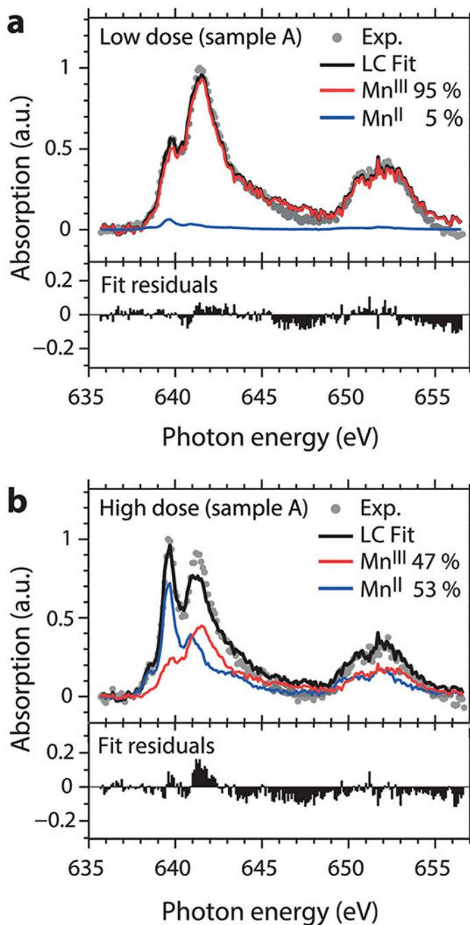
**Fig.4.** Fits (black) of normalized low-dose (a) and high-dose (b) absorption spectra (circles, taken from Fig. 2a) with linear combinations of damage-free spectra of Mn<sup>II</sup>(acac)<sub>2</sub> (blue) and Mn<sup>III</sup>(acac)<sub>3</sub> (red) from ref. 15. Fit residuals are shown in the bottom panels.
