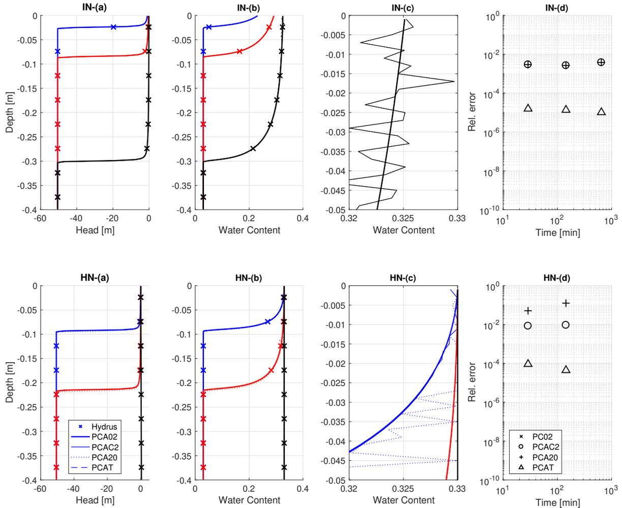
Figure 7: (a): Head and (b): water content profiles for IN and HN scenarios. Blue:  $t = 28$  min, Red:  $t = 144$  min, Black:  $t = 648$  min. The Hydrus results are plotted at coarser resolution for readability. (c): Zoomed water content profiles to show details near the saturated-unsaturated interface. (d): Relative difference in water content ( $\epsilon_\theta$ ) for the tested scenarios (taking PCA02 as the reference solution).
