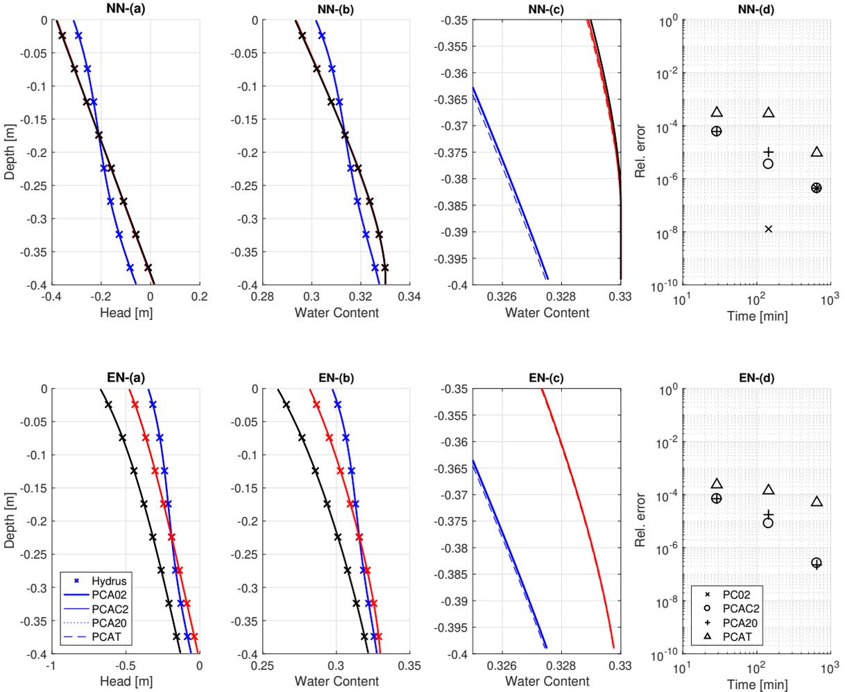
Figure 6: (a): Head and (b): water content profiles for NN and EN scenarios. Blue:  $t = 28$  min, Red:  $t = 144$  min, Black:  $t = 648$  min. The Hydrus results are plotted at coarser resolution for readability. (c): Zoomed water content profiles to show details near the saturated-unsaturated interface. (d): Relative difference of water content ( $\epsilon_\theta$ ) for the tested scenarios (taking PCA02 as the reference solution).
