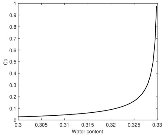
Figure 2: Courant number as a function of water content for the soil given in Table 2. The Courant number is estimated at  $\Delta t = 100$  s.
