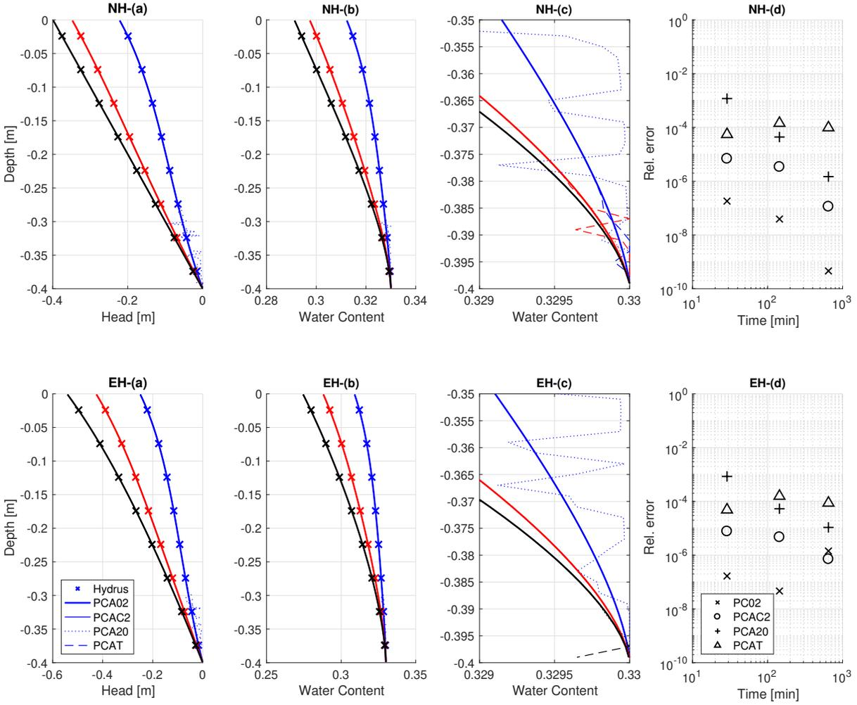
Figure 8: (a): Head and (b): water content profiles for NH and EH scenarios. Blue:  $t = 28$  min, Red:  $t = 144$  min, Black:  $t = 648$  min. The Hydrus results are plotted at coarser resolution for readability. (c): Zoomed water content profiles to show details near the saturated-unsaturated interface. (d): Relative difference in water content ( $\epsilon_\theta$ ) for the tested scenarios (taking PCA02 as the reference solution).
