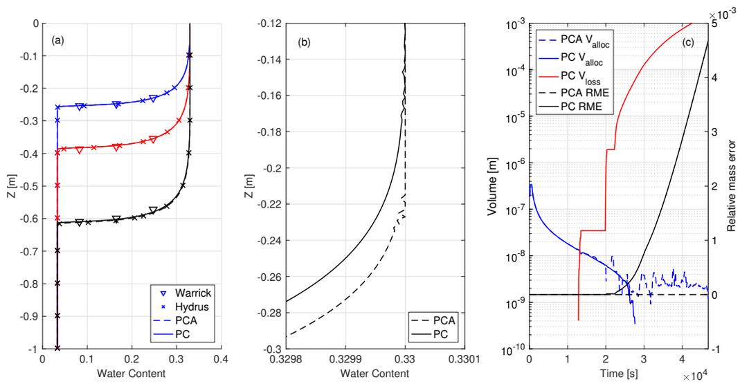
Figure 5: (a): Water content profiles for the Warrick problem with  $\Delta z = 0.2$  cm,  $\Delta t_{\max} = 0.2$  s. The Hydrus results are plotted at a coarser spatial resolution for readability. Blue: 11700 s, Red: 23400 s, Black: 46800 s. (b): Same profiles but zoomed to the saturated-unsaturated interface. (c): Blue: Volume changes during post-allocation, Red: Volume loss for P-C method. Black: Relative mass error (Eq. 20).
