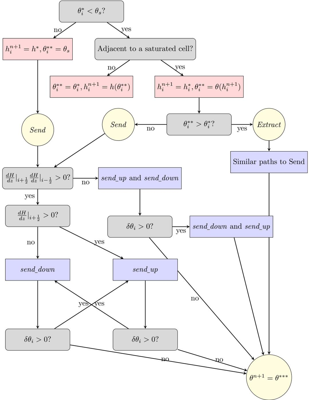
Figure 1: New post-allocation flowchart. *send<sub>down</sub>* and *send<sub>up</sub>* are functions that send excess moisture to nearby cells (see Algorithm 1). The *Extract* operations are similar to *Send*, so they are not expanded in detail. 10
