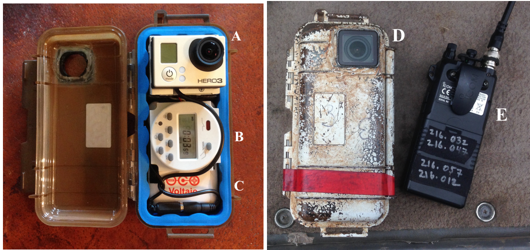
Figure 1-1. Left: CowPro internals including (A) GoPro® HERO3 Black camera, (B) Cam-Do programmable scheduler, (C) Voltaic battery and SwiTronix USB battery eliminator. Right: External CowPro components including (D) customized Pelican Micro 1030 case, (E) Icom IC-R10 wideband receiver.
