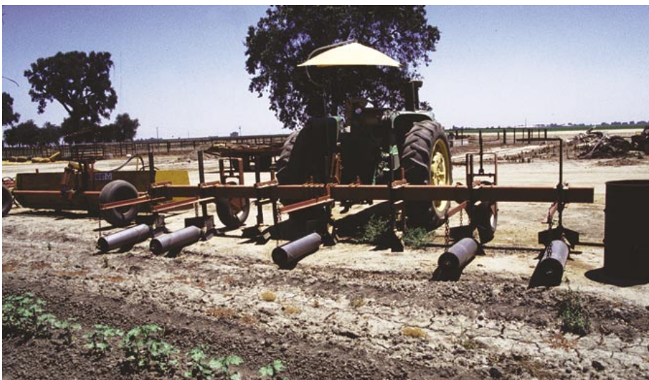
Furrow torpedoes are attached to a sled to ease turning at the end of the field.
