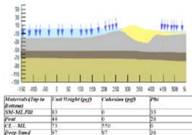
Figure 6. Soil Profile of Existing Levee (Harvey 2010).
