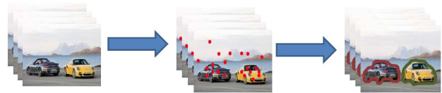
Figure 1. A simple illustration of the proposed problem. Given a video sequence (left), we collect eye tracking data in the sequence from multiple subjects (center) and utilize this information to extract visually salient objects (right). Best viewed in color.
