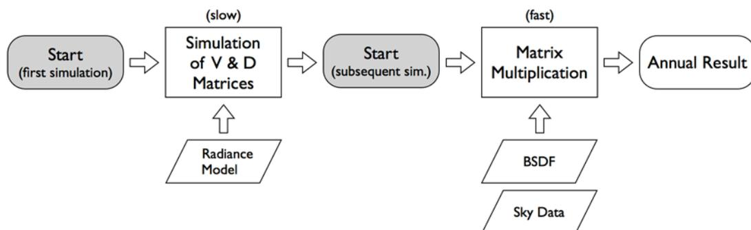
**Figure 1.** Simulation process flow chart
