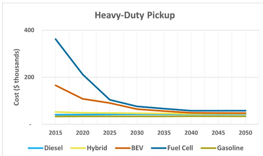
Figure 5-8. Capital cost of heavy-duty pickup trucks through 2050.
