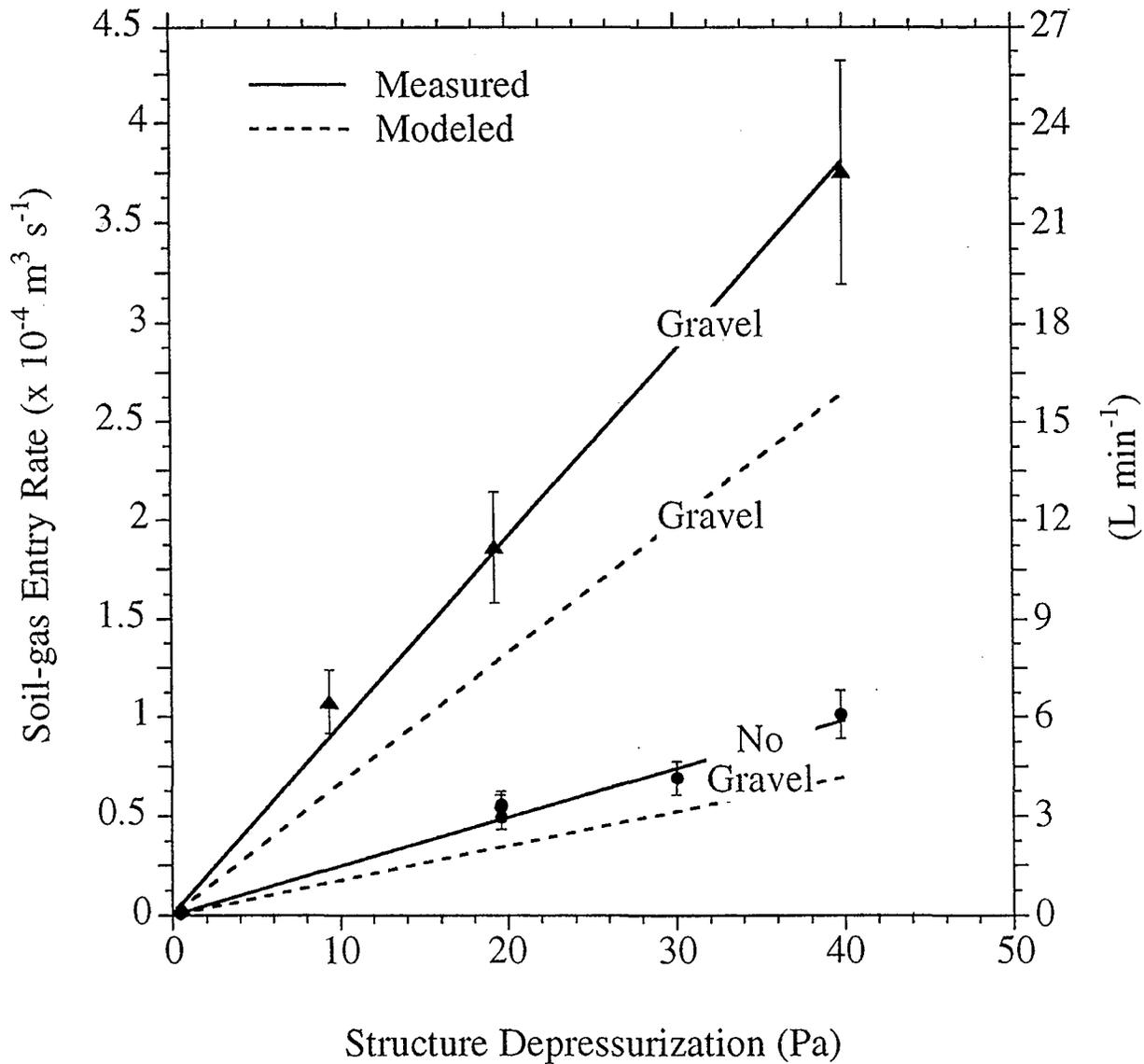
Fig. 2. A comparison of measured and modeled soil-gas entry rate into both structures as a function of structure depressurization. Lines through measured points are linear regressions weighted by uncertainties. The vertical bars represent measurement uncertainty.
