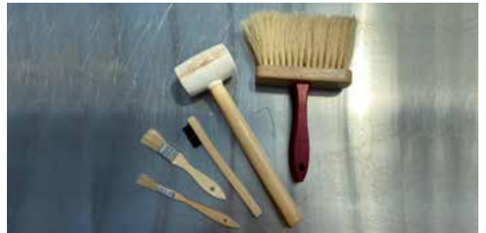
FIGURE 18. Brushes and mallet to clean vacuum seeder, eliminate doubling, and sweep seed to fill gaps on seed plate. Photos: Christof Bernau
