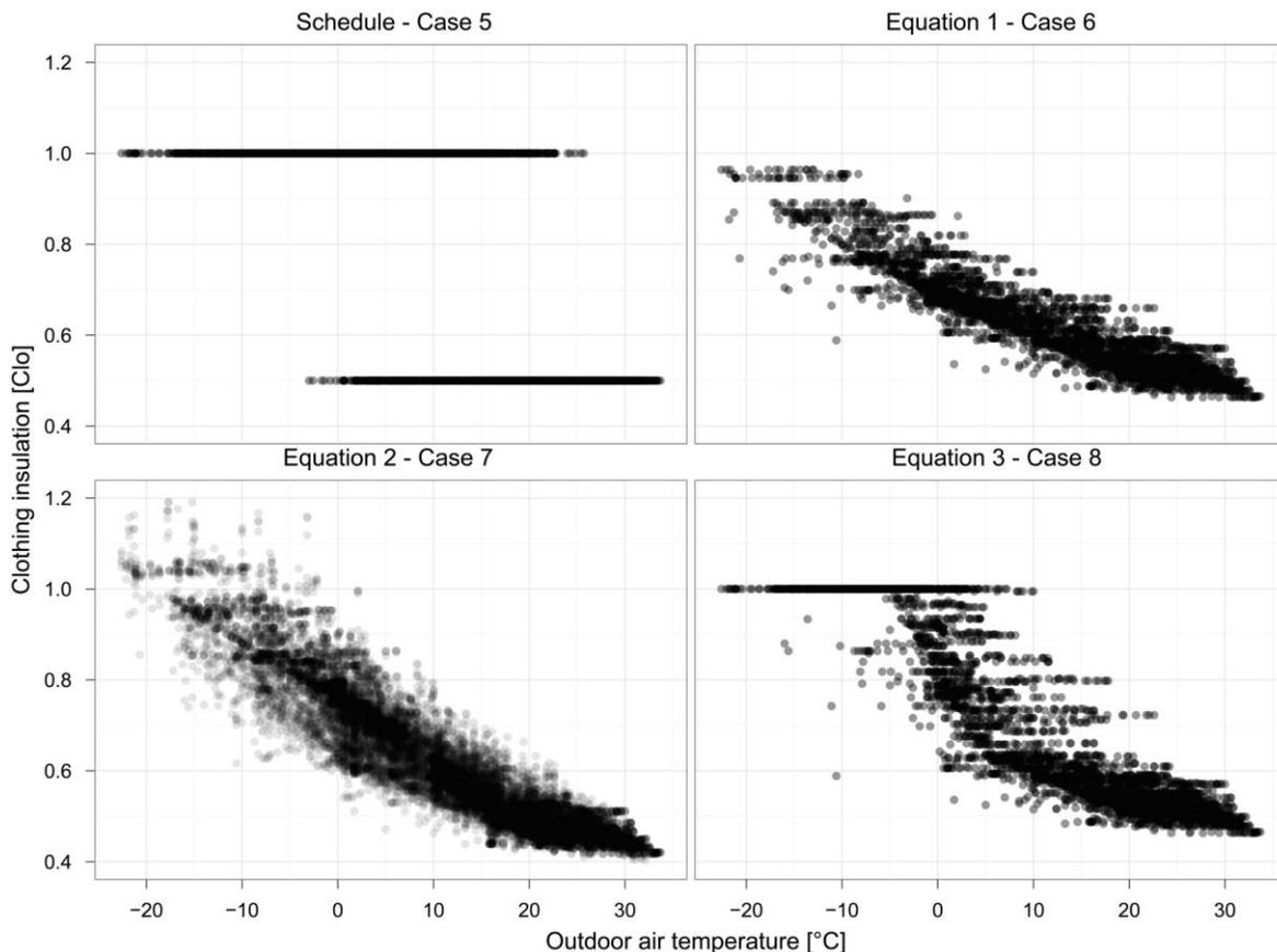
Figure 5. Outdoor air temperature vs. clothing insulation for Cases 5 (Schedule), 6 (Eq. 1), 7 (Eq. 2) and 8 (Eq. 3).
