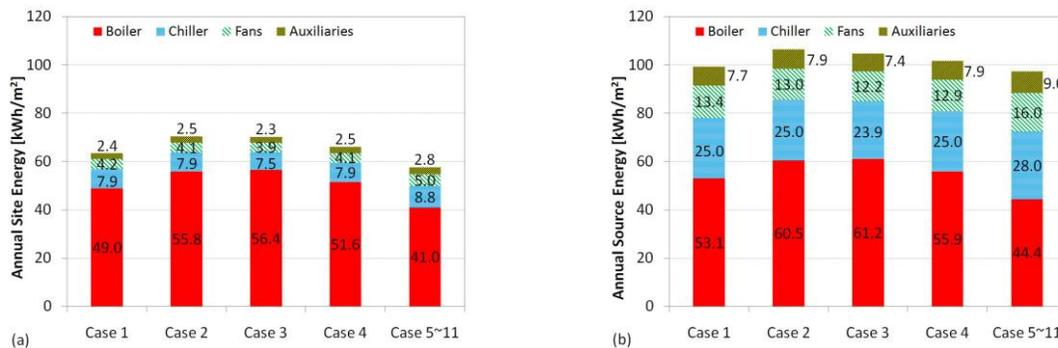
Figure 6. Annual energy breakdown (boiler, chiller, fans, auxiliaries) for (a) site and (b) source – primary energy.
