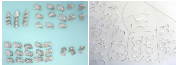
FIGURE 4. DRILLING AND MILLING CHIPS SORTED BY SIZE AND SHAPE.
