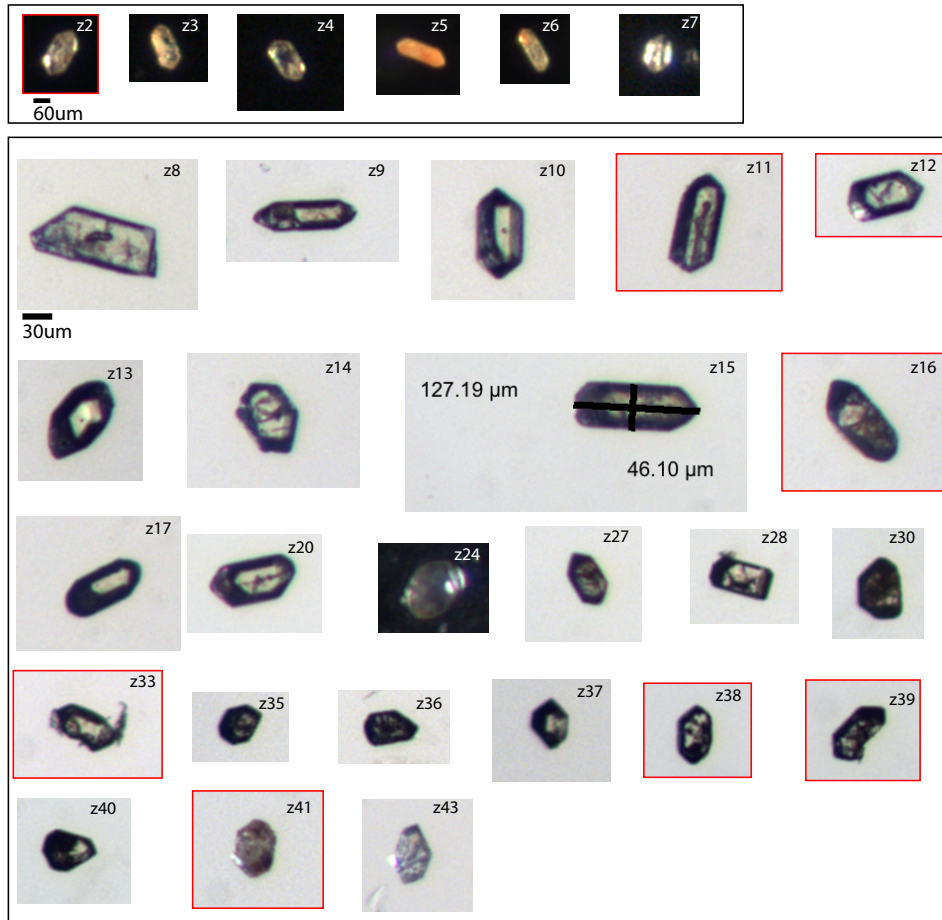
Figure 8. Photomicrographs of zircon grains from samples SAM-ET-04. Grains with a red border were used for the weighted mean age.
