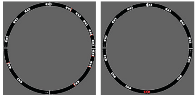
Figure 1 Left: Vehicles not equipped with flow smoothing technology will quickly form stop-and-go traffic waves caused by vehicles braking and then accelerating too much. Right: Introducing a flow-smoothing AV (red car) stabilizes vehicle speeds, primarily by maintaining a gap between the vehicle it is following.
