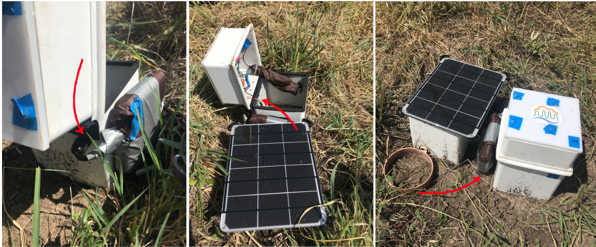
Figure A.6: Red arrows pointing to the USB connection through the through-port gland (left) connecting the electronics (middle) to the external, waterproofed battery (right). The round PVC collar used for paired CIRAS data collection is visible in the right panel.
