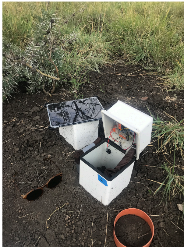
Figure 3.3: A fluxbot installed in the field, in its open position, with actuator fully extended. Collar for manual data collection at bottom right.
