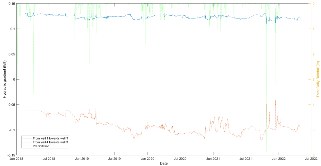
Figure 4: Hydraulic gradient between well 3 and other wells over time.
