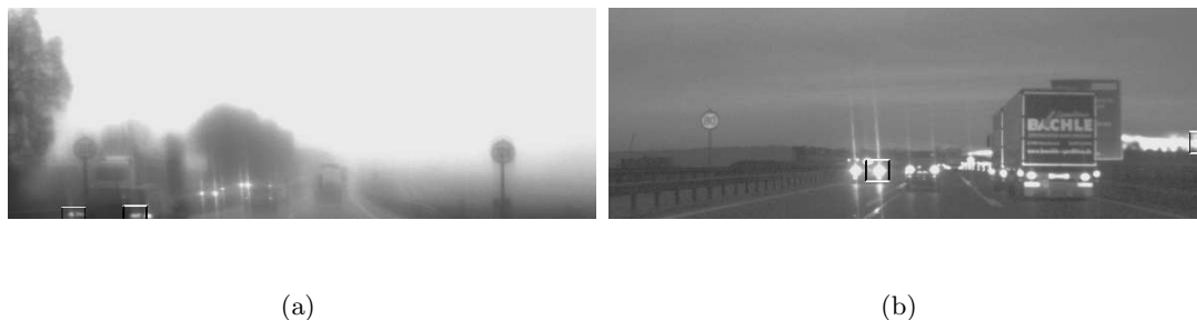
Figure 5.6: Missed speed-limit signs due to low overall contrast in the scene. Note the bright oncoming headlights and saturated white highlights from the sun at the horizon.
