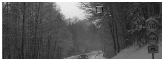
Figure 5.8: Speed-limit sign in a snowy setting that has been significantly occluded. The main characteristic (the red border around the sign) has been covered with ice and presents a difficult detection and recognition case.
