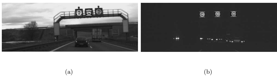
Figure 5.4: Digital speed-limit sign detection. (a) Highway scene with a successfully detected overhead digital sign. (b) Highway scene at night with all three displays detected.
