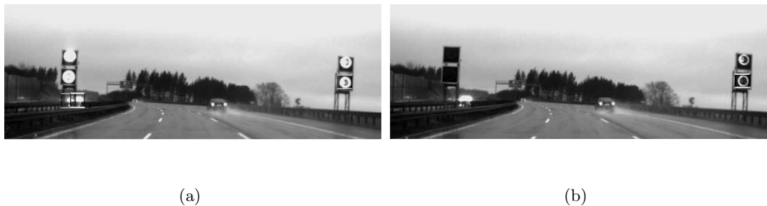
Figure 5.7: Digital sign frequency with camera-capture rate synchronization occurrence can be seen in the two consecutive frames above. (a) All four digital displays are lit and allow for detection. (b) The two displays on the left appear completely off while the right ones are in the process of flashing off and appear dim.
