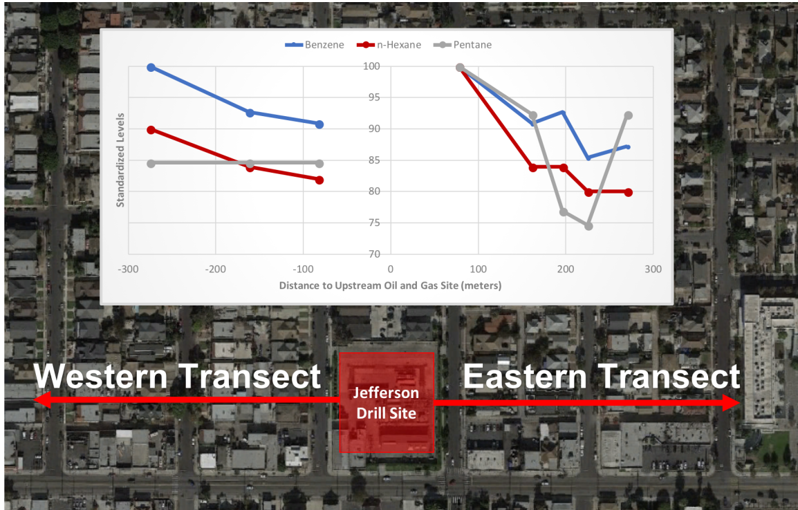
Figure 3.2: Transect through the Jefferson drill site and results of the distance decay gradient for data collected between February 17 – March 2, 2016.
