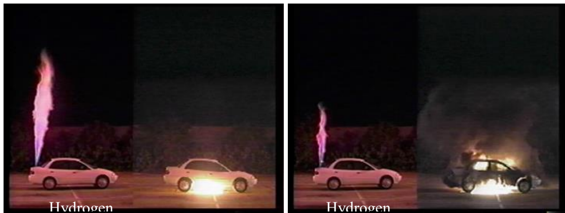
Figure 20 Fuel leak and fire test with hydrogen vs. gasoline fuel (Swain, 2001)
