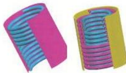
Figure 16 Heat exchanger: tube wrapped round engine jet pipe (Westenberger, 2003)
