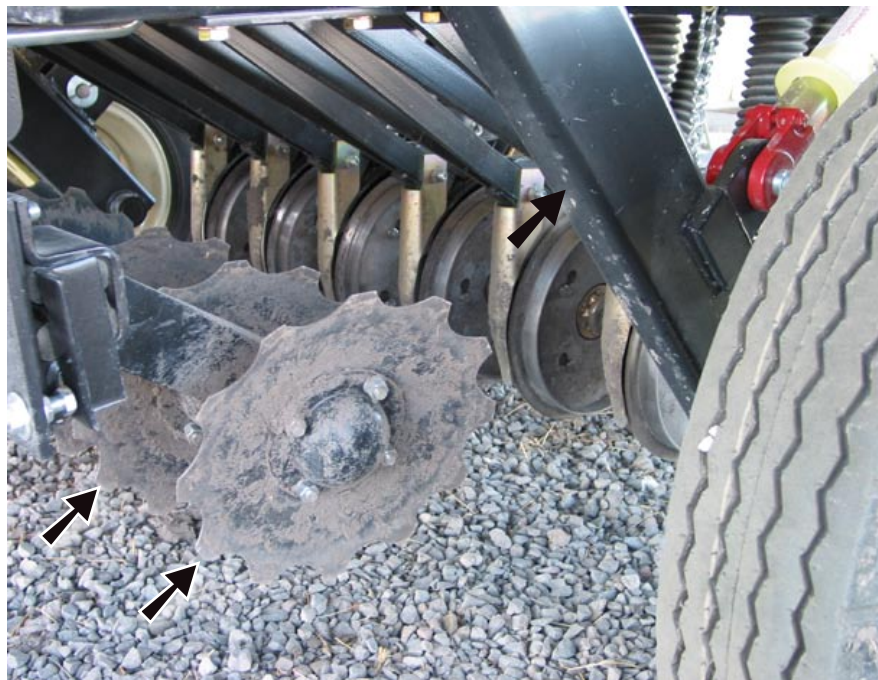
Trash coulters mounted in front of the double-disk opener on a no-till drill. Trash coulters cut through sod and litter to achieve proper seed placement in the soil.
