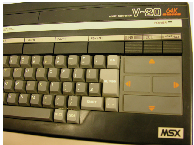
Figure 2. The MSX was a hybrid console-computer, popular in Japan in the mid-1980s. Though it looked much like other personal computers of the time, its standardized cartridge format and graphics acceleration made it attractive to game developers. (Photo by Paolo Tonon.
