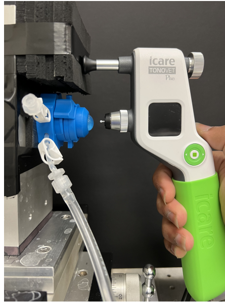
Figure 5.1. Setup for testing with the commercial tonometer (TonoVet Plus).
