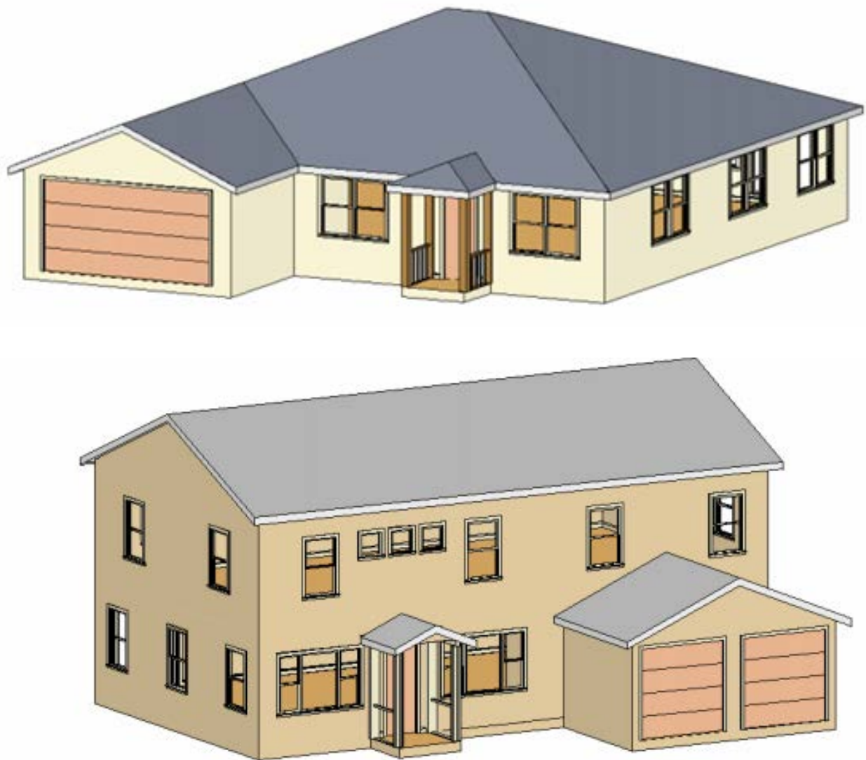
Figure 2. Rendering of two prototype homes simulated: a 1-story 2,100 ft 2 (195 m 2 , top) and a 2-story 2,700 ft 2 (251 m 2 , bottom)
