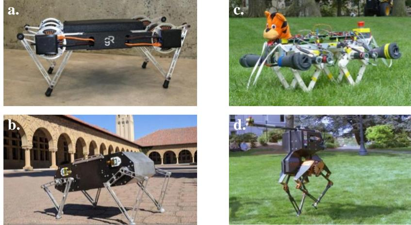
**Figure 1.1:** A class of small robot that use planar 5-bar linkages design, capable of compliance control through direct or quasi-direct drive motors. a) Ghost Robotics Minitaur [17]. b) The Stanford Doggo [18]. c) MIT Mini Cheetah [19]. d) The T Robot [20].
