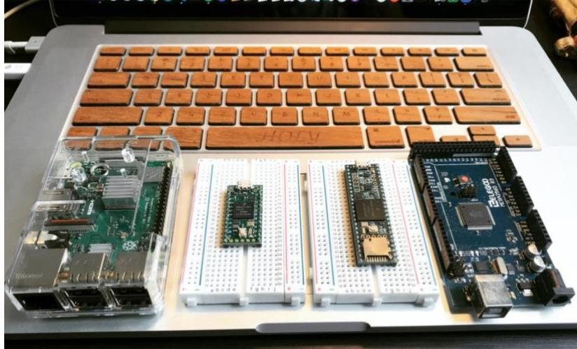
**Figure 3.3:** Popular microcontrollers for medium-small size robots. Besides a laptop, a small size and high-speed controller might also be a perfect choice to perform agile and accurate locomotion in most robotics research. Starting from the left: RaspberryPi 3b, Teensy 4.0, Teensy 3.5 and Arduino Mega 2560.
