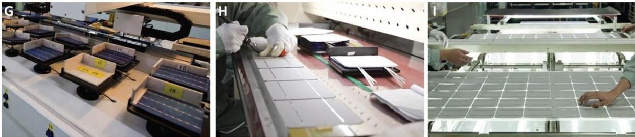
**Figure 3.2. Process flow of making c-Si PV modules.** The images in A-I are representative for key steps in the process flow: surface texturing (A), furnace doping (B), edge isolation and PSG removal (C), passivation and anti-reflection coating (D), screen printing (E), contact firing (F), testing and binning (G), stringing cells (H), and lamination (I). Image courtesy: Q-Cells [74] and Suntech [75].
