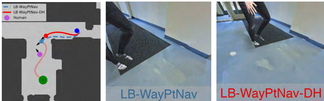
Figure 7.13: (left) The robot starts at the dark blue circle. Its goal is to move to the green goal region without colliding with static obstacles (dark gray) or humans (magenta). LB-WayPtNav follows the light-blue, dashed trajectory until the light blue dot, planning a path to the right of the human (in its direction of motion), leading to collision. LB-WayPtNav-DH follows the red trajectory until the red circle, planning a trajectory (transparent red) to the left of the human which accounts for its future motion, and ultimately leads to success. (middle & right) Corresponding RGB images seen by the robot.
