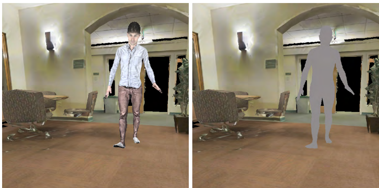
Figure 7.16: LB-WayPtNav-DH trained on images from HumANav with realistic textures (clothing, hair, skin color, facial features) (left) leads to a better generalization than training on human figures with gray textures (right).
