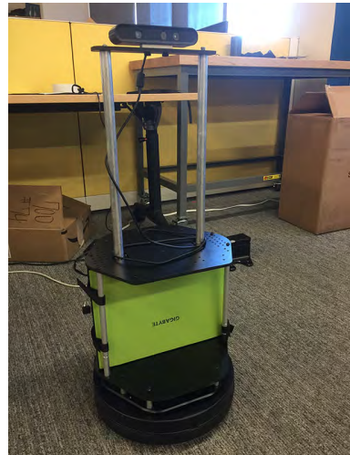
Figure 7.7: Our Turtlebot 2 hardware platform uses a Yujin Kobuki base, Gigabyte Aero Laptop, and Orbbec Astra camera.
