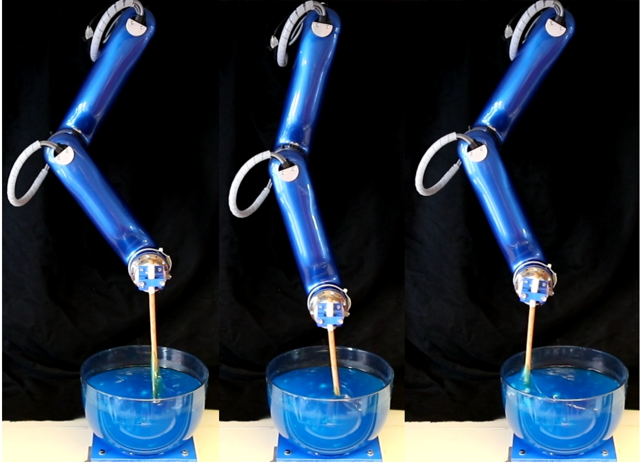
Figure 6.12: Stirring viscous liquid with the 3-dof SCARA robot CARBO using aDOBO.
