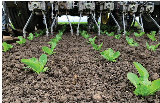
Figure 7. Automated weeder with split blades that can weed in the seedline in between crop plants.
