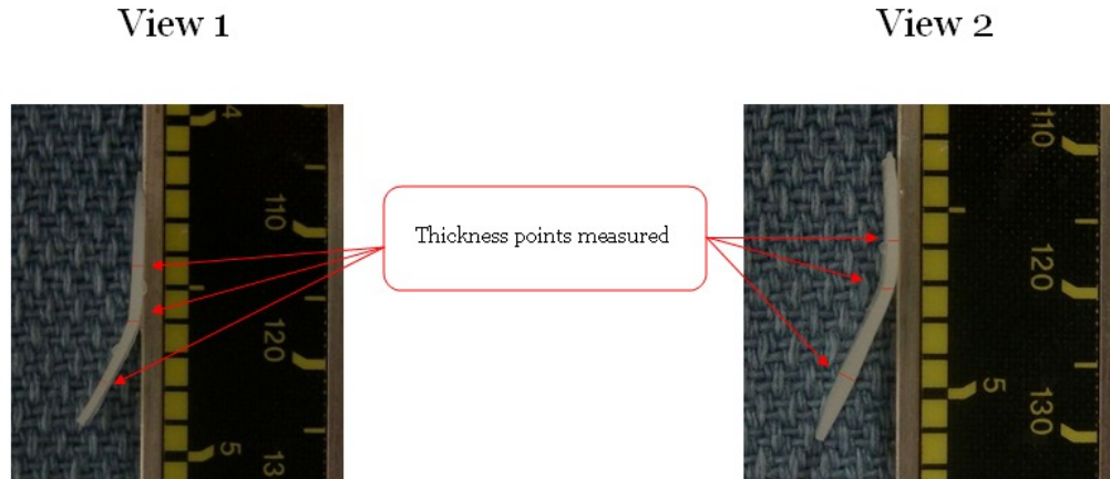
Figure 7. Photographs of both sides of the same cartilage specimen are taken. For each side, the midpoint, maximum, and minimum thicknesses are measured and averaged.
