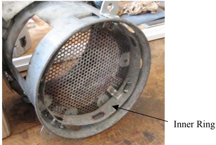
Figure 3: Inner ring to block a direct air path through the primary air holes.
