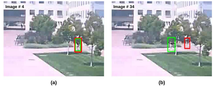
Fig. 1. Two frames (a) and (b) of a sequence with a pedestrian walking from right to left. The red and green boxes represent the tracker's predicted object location and ground-truth, respectively. Typical appearance-based trackers fail on such low visual-quality video sequences.
