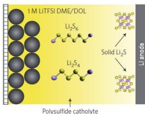
Figure 1. A scheme of Li-S batteries illustrating working mechanism and the shuttle effect. Figure reproduced from Reference 4.
