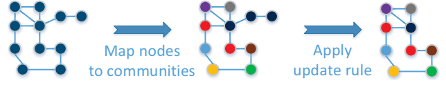
Figure 3: Updating graph structures by mapping nodes to detected communities and applying the merging rule. (Left) represents the initial graph representation as described in Section 2.1. (Middle) Each color represents an updated representation for each node using the concept of communities. (Right) The final updated graph representation with adjacent nodes of same color merged. Figure is best viewed in color.
