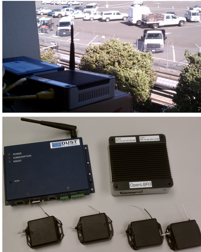
Figure 2.9: Long-term deployment setup at the Chevron-Richmond refinery. The result of this test was a detection rate of 100% with no false alarms. The sensors withstood strong winds and rainy weather.
