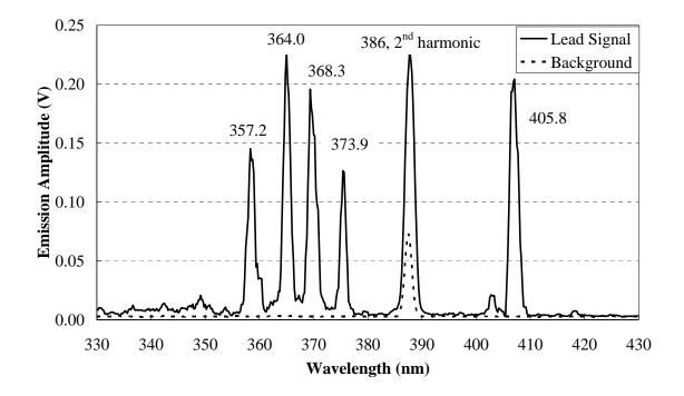
Figure 3: Time resolved emission from  $Pb(NO_3)_2$  (405.8 nm) and background (415 nm) at various fluence conditions. (a) Emission during the first  $\mu$ second.
