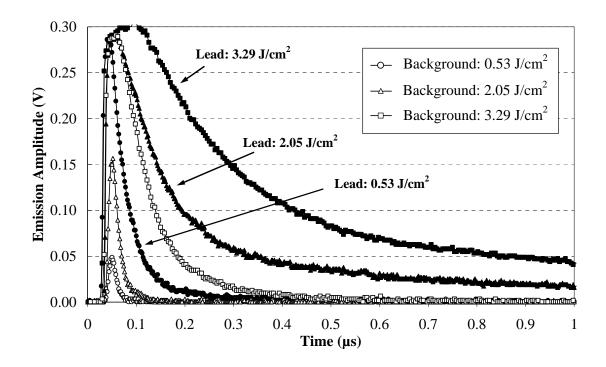
(b) Lead emission at longer time scales. Note that plasma formation threshold appears approximately  $2 \text{ J/cm}^2$ .
