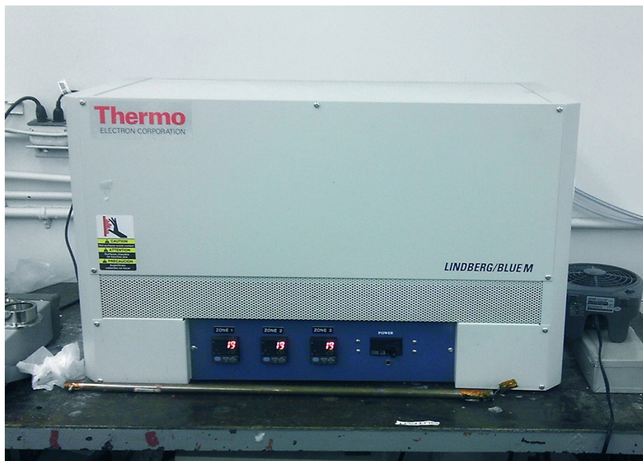
Figure 3.6 Photograph of the Lindberg/Blue M three-zone tube furnace that was used for H 2 sensing tests.
