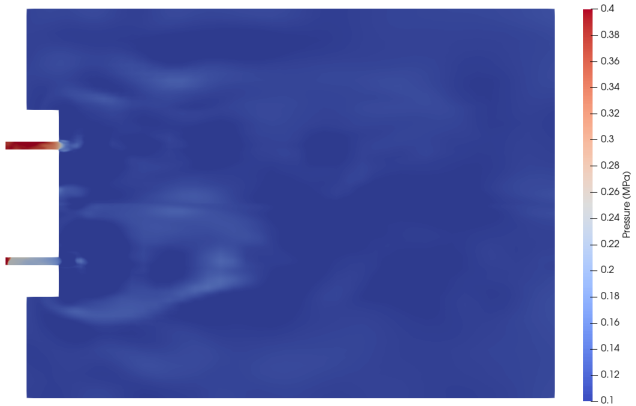
Figure 3.13: Snapshot of pressure in the exhaust at a simulation time of 5.08 ms from simulation start, 1.18 ms from being manually set to 0.12 MPa.
