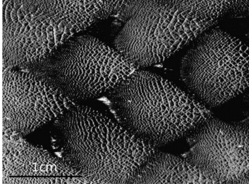
Figure 1.4: Soot foil showing a double-cellular structure from the passage of a detonation in a \text{H}_2 - \text{NO}_2/\text{N}_2\text{O}_4 mixture, from Joubert et al. [25].
