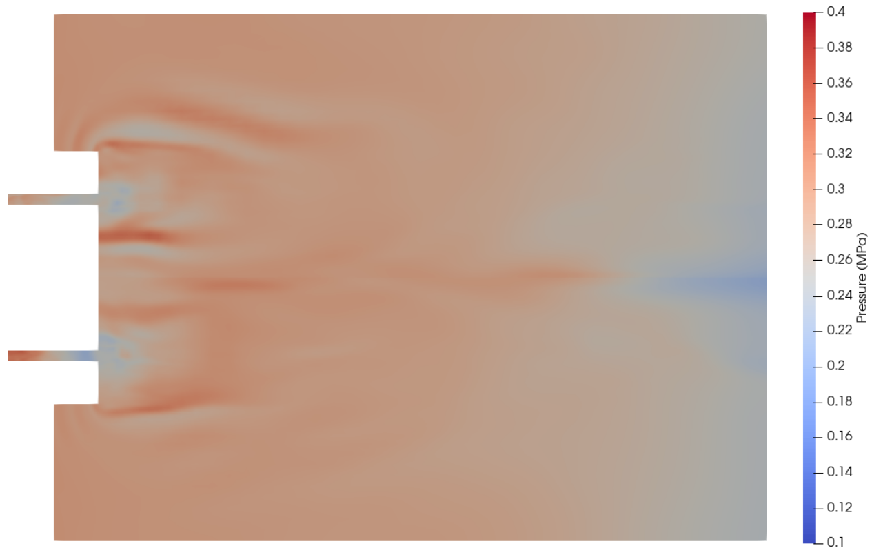
Figure 3.10: Snapshot of exhaust pressure, taken at the end of the cascade process, 2.75 ms after simulation start.
