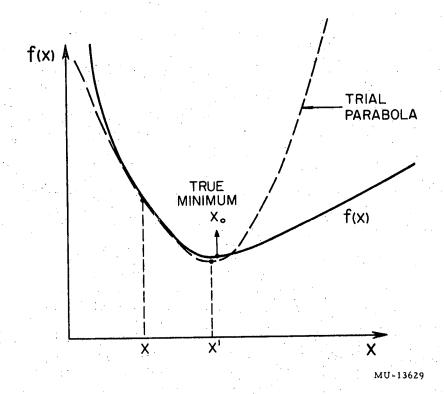
Fig. 1. Example of a trial fit by the parabolic method. The solid curve is the true function. The dotted curve is the trial parabola to the point x. x' is the minimum of the trial parabola and is the new trial point.
