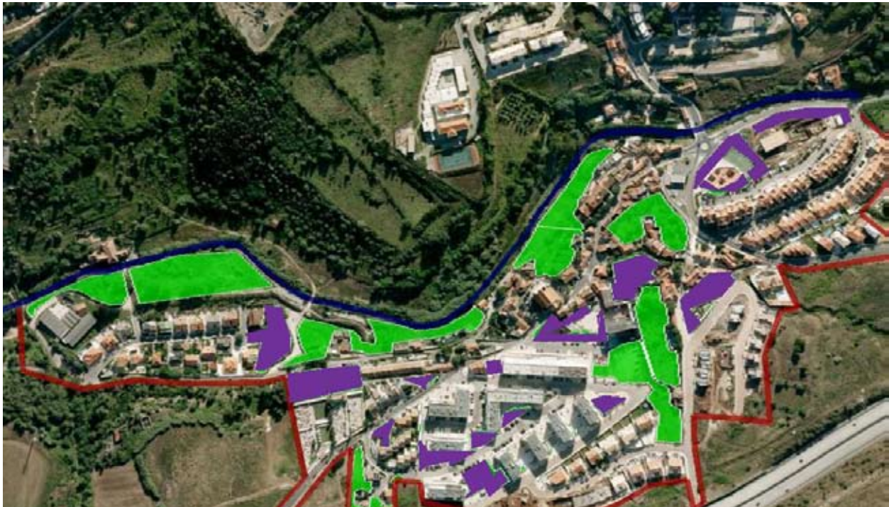
Rain garden opportunity sites in Barcarena (purple) and existing pervious vegetated sites (green).
