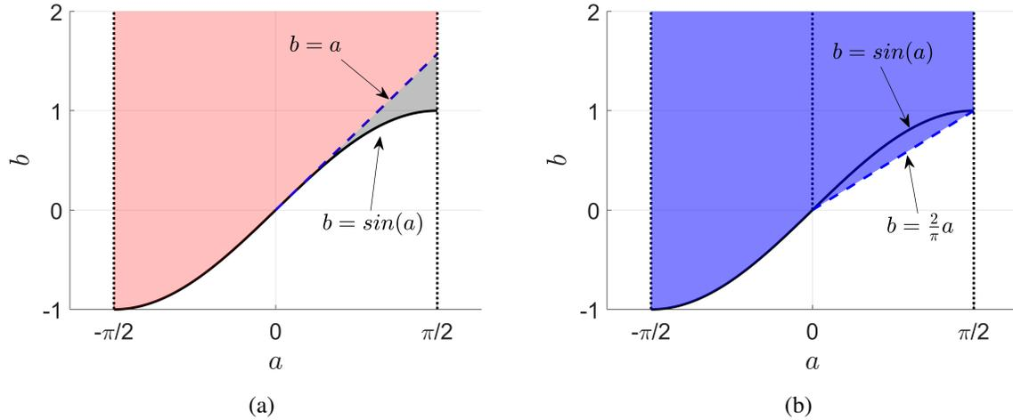
**Figure 4.1:** Tightening and relaxation of a sinusoidal non-convex constraint. In plot (a), within  $|a| < \pi/2$ , by ignoring the gray region delimited by  $b = a$ ,  $b = \sin(a)$  and  $a = \pi/2$ , the non-convex set characterized by  $\sin(a) \leq b$  appearing in (4.20a) contains the red convex subset  $\mathcal{H}^+$ . On the other hand, in plot (b), this non-convex set is contained in the blue region. Each of the blue regions separated by the dotted line at  $a = 0$  are convex.
