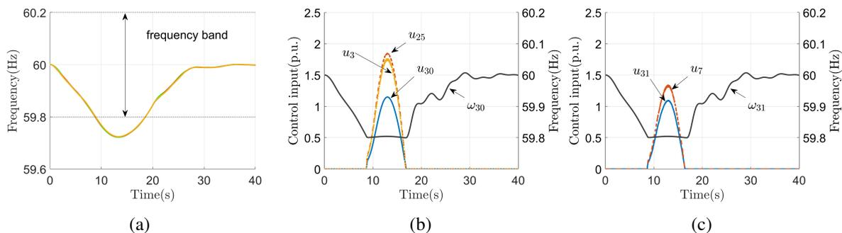
**Figure 5.2:** Plot (a) shows the frequency trajectories of generators 30 and 31 without the controller, going beyond the lower safe frequency bound. With the centralized controller, plot (b) and (c) show the trajectories of the control inputs and frequency within each region.
