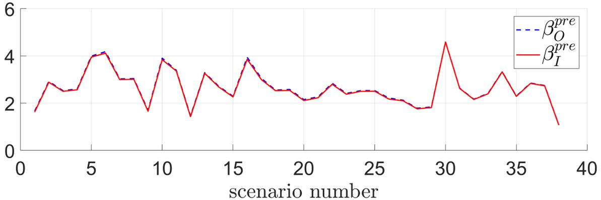
**Figure 3.8:** Robustness characterization of the IEEE39 bus network based on tolerableness sets. In each scenario, we inject a disturbance at the corresponding node and compute the approximations of the robustness metric defined in Remark 3.3.8. This metric measures the maximum allowable disturbance that does not violate transient safety. Both approximations use 301 sampling points optimized through Algorithm 1.
