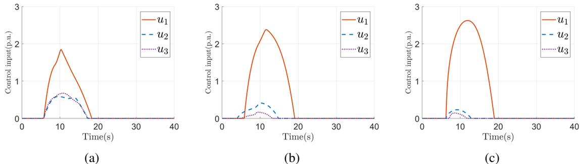
**Figure 5.5:** Input trajectories of controlled generators in IEEE 9-bus example under (a) centralized controller, (b) distributed controller, and (c) controller proposed in [ZC19c]. All of them guarantee stability and frequency invariance.
