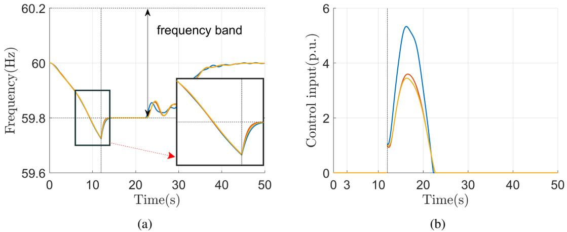
**Figure 4.7:** Frequency and control input trajectories with transient controller available after  $t = 12$ s. Plot (a) shows the frequency trajectories of generators 30, 31, and 32. Due to the disturbance, and without the transient controller, all 3 frequency trajectories exceed the 59.8Hz safe bound at  $t = 12$ s. As the transient controller kicks in, the unsafe trajectories come back to the safe region and never leave afterwards. Plot (b) shows the control input trajectories.
