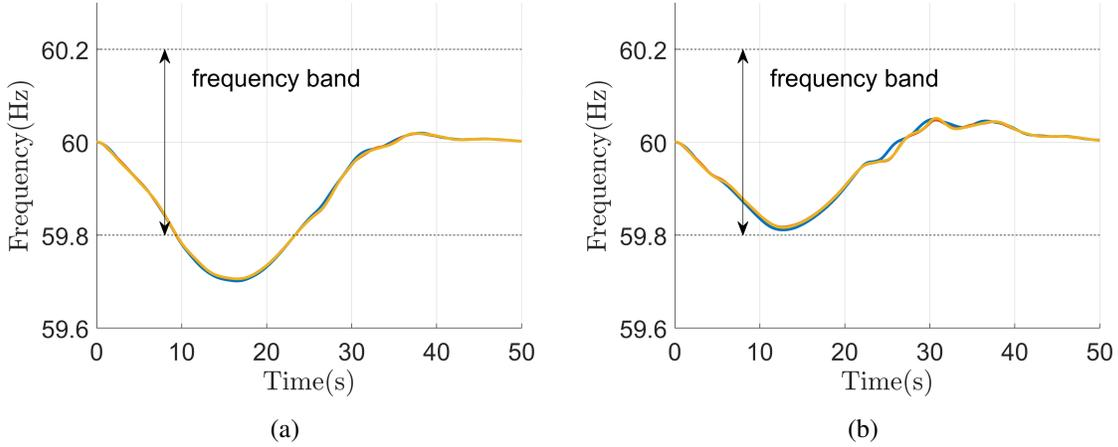
**Figure 4.4:** Frequency trajectories under non-ideal actuator dynamics. Plot (a) shows the frequency trajectories of generators 30, 31, and 32 with the control command (4.10) as the setpoint of a first-order actuator. Plot (b) shows the same but with the control command (4.10) implemented with tighter safe frequency bounds.
