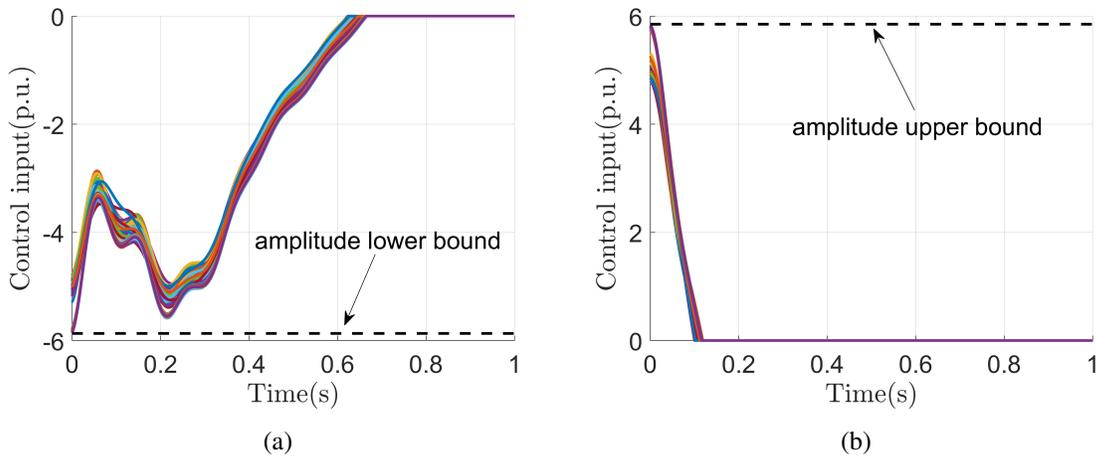
**Figure 4.8:** Control input trajectories at node 30 corresponding to 100 different initial states. In plot (a), with all initial states randomly selected around the worst-case scenario, all 100 trajectories are lower bounded by  $-5.8686$  (denoted by the dashed line), as guaranteed by Lemma 4.4.4. A similar result is illustrated in plot (b), where another 100 trajectories with random initial states are upper bounded by  $5.8494$ .
