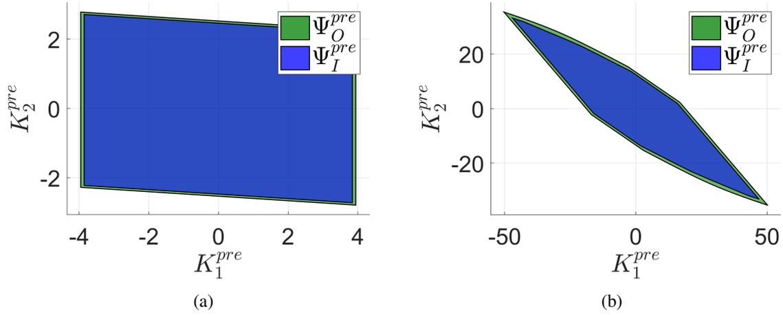
**Figure 3.5:** Inner and outer approximations of transient-state tolerableness set for the precisely known case with different trajectory forms. In plot (a), the trajectory form is  $\zeta^{pre}(t) = [1(t - 1s) \ 1(t)]^T$  and in plot (b)  $\zeta^{pre}(t) = [\sin(\pi t) \ \sin(\pi t)]^T$ , respectively.
