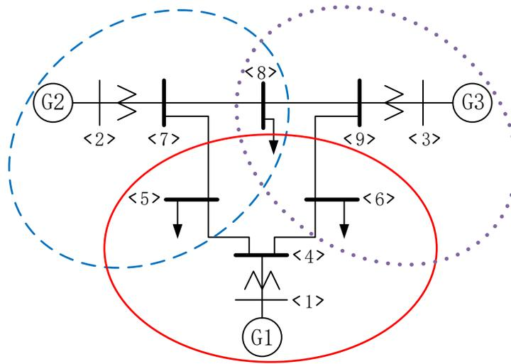
**Figure 5.4:** IEEE 9-bus power network with network partition.
