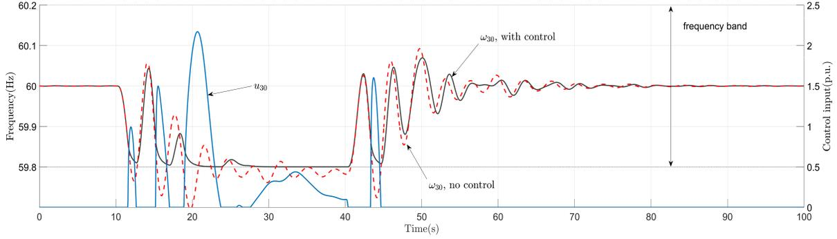
**Figure 4.2:** Frequency and control input trajectories at node 30 corresponding to the power supply loss of generator G9 during [10,40]s. The frequency trajectory without transient controller goes beyond the safe bounds during the contingency, while this is avoided with the proposed controller. Notice that the latter only takes effect when the frequency is close to the safe bound.
