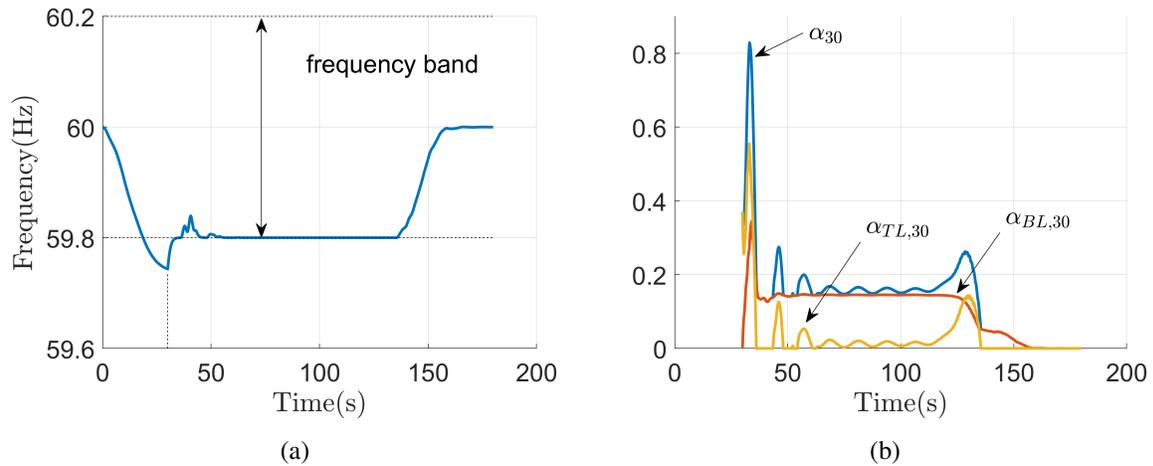
**Figure 6.5:** Frequency and control input trajectories at node 30 when the controller is only turned on after 30s. In plot (a), the frequency gradually comes back to the safe region once the controller kicks in. Plot (b) shows the control signals.
