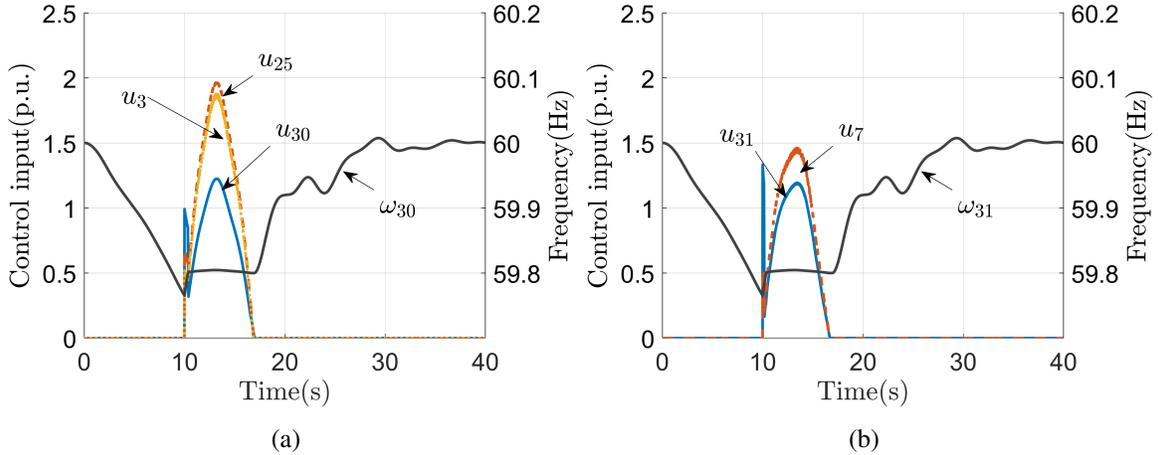
**Figure 5.3:** Frequency and control input trajectories with centralized controller available only after  $t = 10s$ , plot (a) for the region with generator 30, and plot (b) for the region with generator 31.
