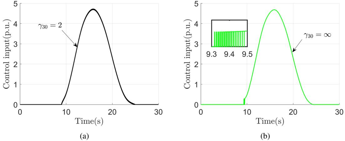
**Figure 4.6:** Control input trajectories at node 30 with linear class- $\mathcal{K}$  function with slope  $\Gamma_{30} = 2$  and  $+\infty$ , respectively, under state measurement errors in  $\omega_{30}$ . The controller with  $\gamma_{30} = 2$  is Lipschitz continuous (cf. plot (a)), whereas the controller with  $\gamma_{30} = +\infty$  (cf. plot (b)) is discontinuous.
