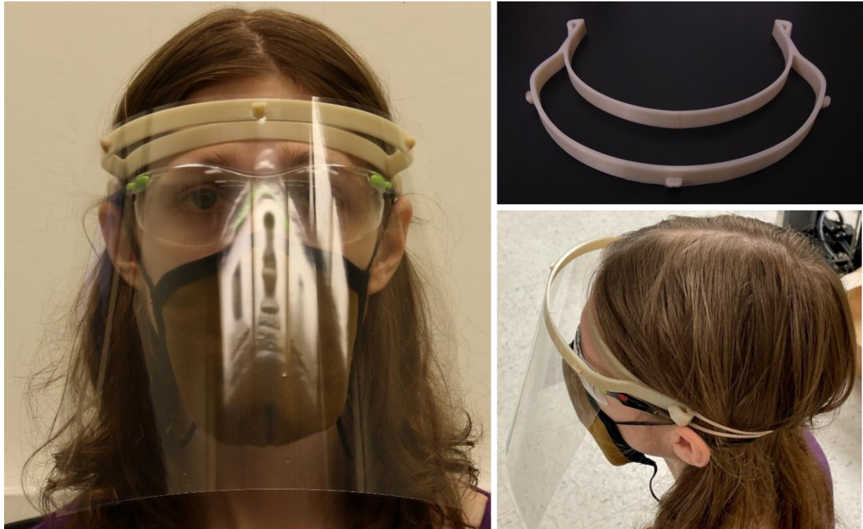
Figure 21: A researcher wearing a face shield 3D printed from CoPA. After autoclaving face shields printed from CoPA there is only a small amount of deformation, and the part remains fully usable.
