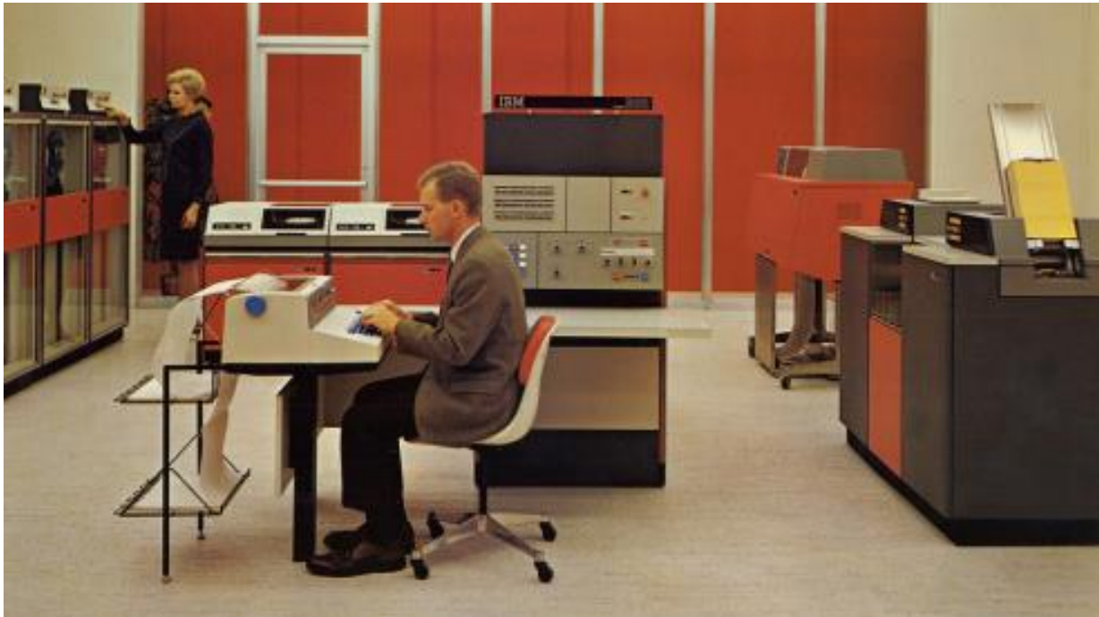
Teletype output device for IBM System 360 mainframe computer.
