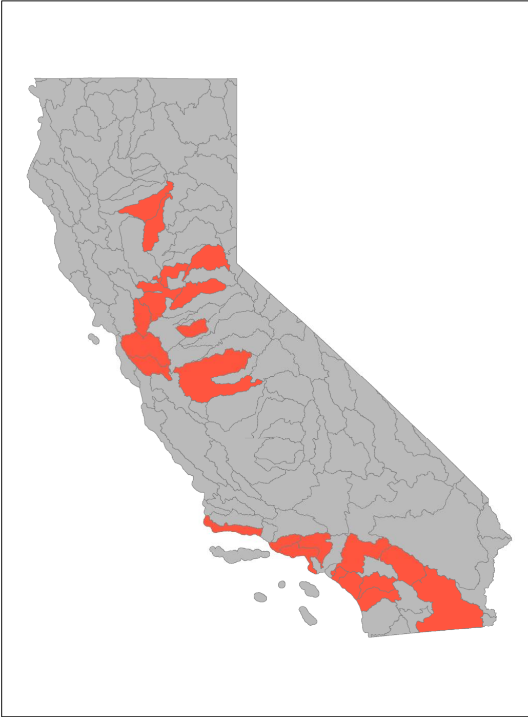
Figure 7: California watersheds that cumulatively receiving higher discharge from effluent than the underlying baseflow.
