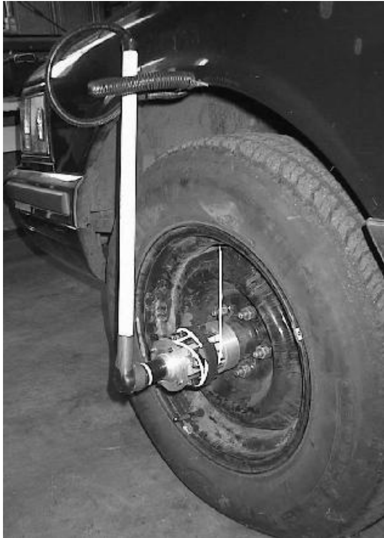
Figure 4.2: Brake torque sensor installed on the Red Towncar.
