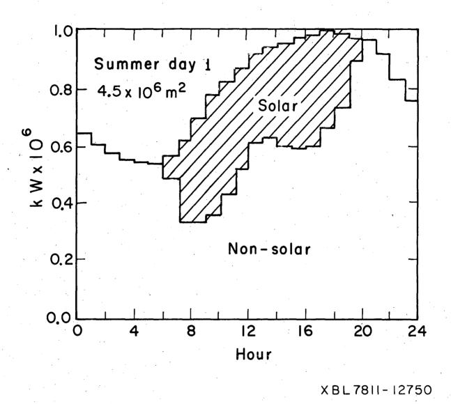
Fig. 2 Solar Contribution to Utility Load - Diurnal Cycle
