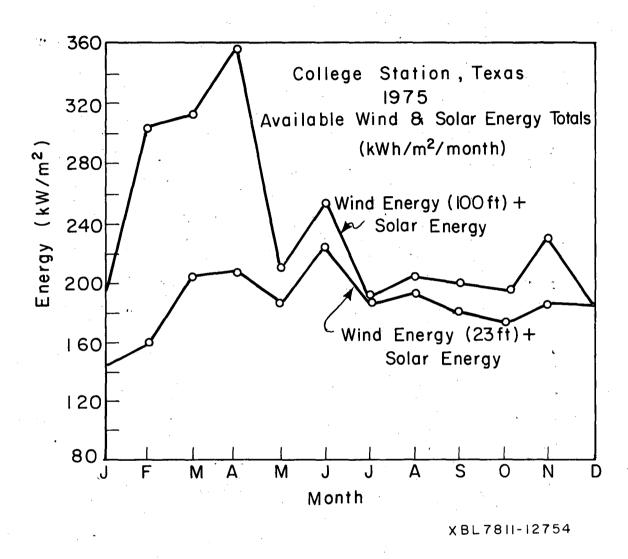
Fig. 4A Joint Wind/Solar Energy Availability
