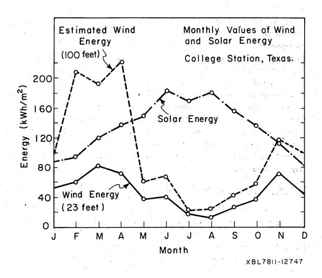
Fig. 4B Joint Wind/Solar Energy Availability
