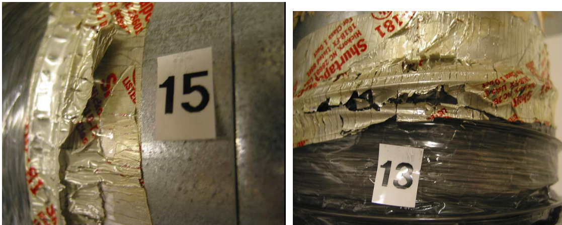
Figure 7. The OPP tape showed considerable visual degradation, even though it still provided a good air seal for the core-to-collar samples.
