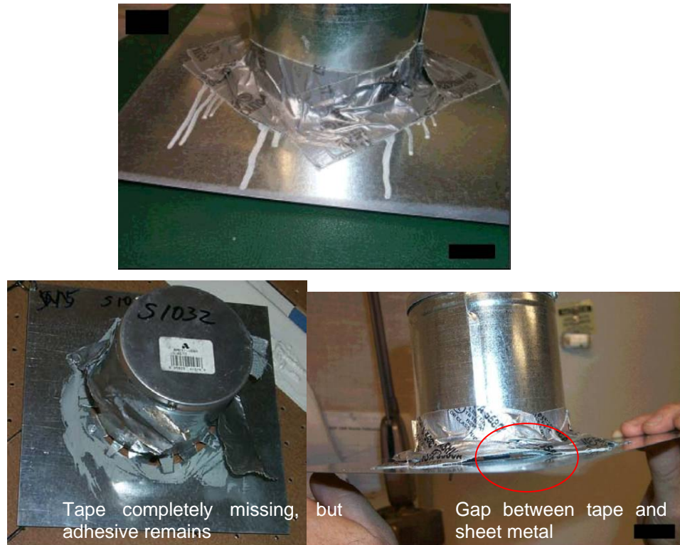
Figure 4. Example failures of the collar-to-plenum joint.
