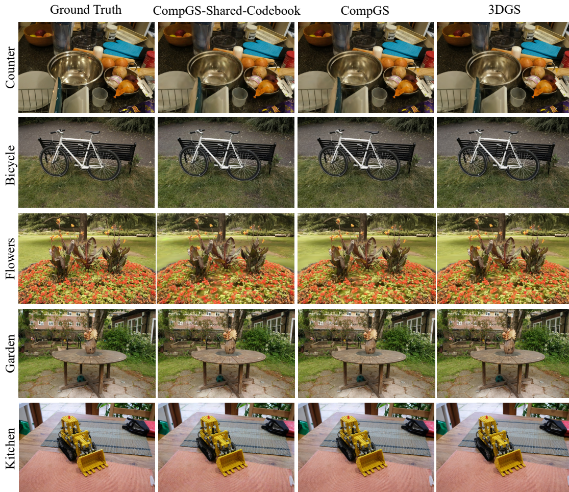
FIGURE B.3. Qualitative analysis of shared codebook. We show the generalization of codebook learned using a single scene on various scenes of the Mip-NeRF360 dataset. The codebook was trained on the ‘Counter’ scene (row-1) and frozen for the remaining scenes. The codebooks for all four parameters (DC, SH, Scale, Rot) are shared across scenes. Both CompGS and CompGS-Shared-Codebook are visually similar to the uncompressed 3DGS with no conspicuous differences between them. 3DGS-No-SH requires twice more memory than CompGS while 3DGS is ten times bigger than CompGS. The scenes and views used for visualization were chosen at random.
