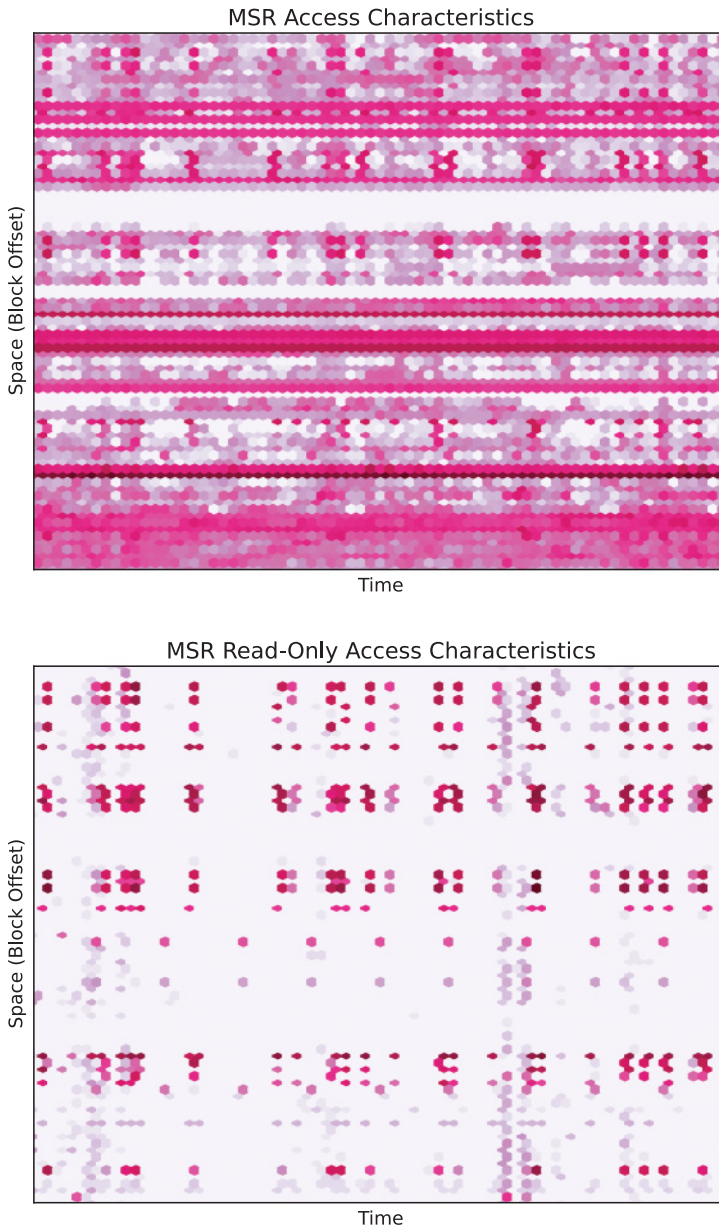
Fig. 8. These 2D histograms show the spatiotemporal layout of block accesses across the msr trace with and without writes. Darker bins correspond to higher access density.
