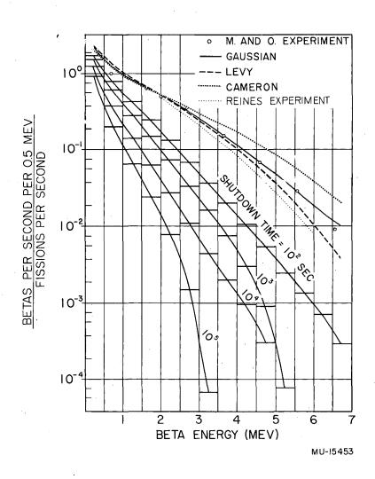
Fig. 2. Energy Spectrum of Betas from  ${\rm U}^{235}$  Fission Products. (Also included is the spectrum as a function of time after shut down of the reactor.)
