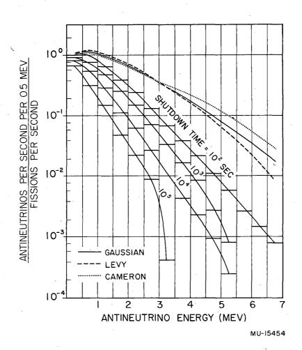
Fig. 3. Energy Spectrum of Antineutrinos from  ${\rm U}^{235}$  Fission Products. (Also included is the spectrum as a function of time after shut down of the reactor.)
